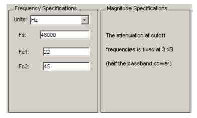
**6** After specifying the filter design parameters, click the **Design Filter** button at the bottom of the design panel to compute the filter coefficients. The display updates to show the magnitude response of the designed filter.
